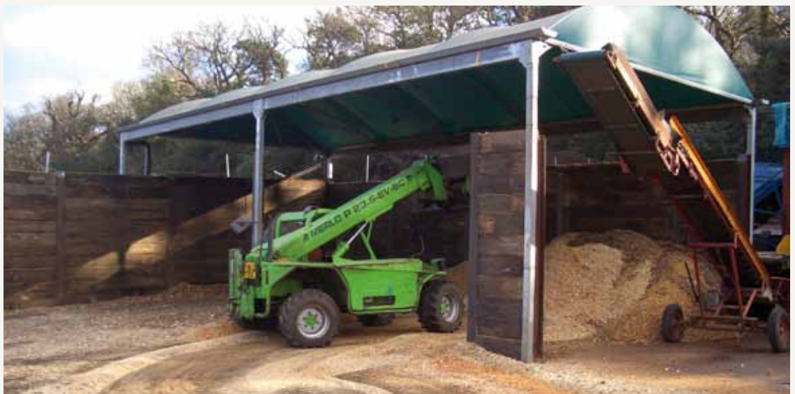
Fuel quality wood chip from tree surgery waste for electricity generation at heat and power stations and for woodchip boilers in municipal buildings. © City Suburban Tree Surgeons Ltd
