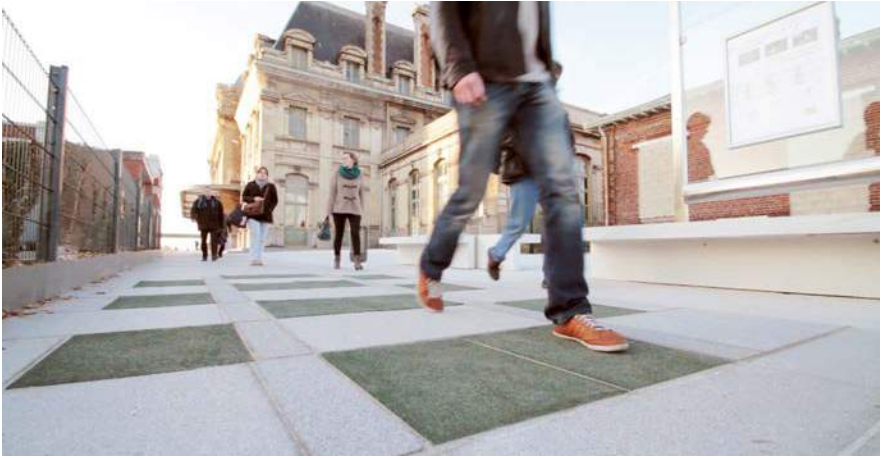
Pavegen's energy-converting tiles harvest energy from pedestrian footfall and transform it into electrical power.
